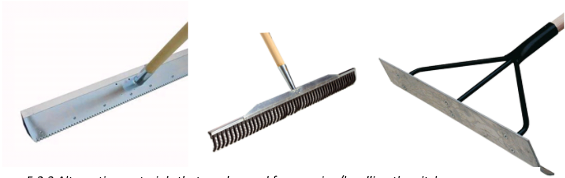
Figure 5.2.3 Alternative materials that can be used for scraping/levelling the pitch.
